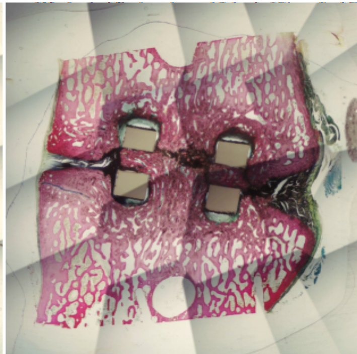
Competitive Ti Plasma Sprayed PEEK Implant: 16 weeks post-op
